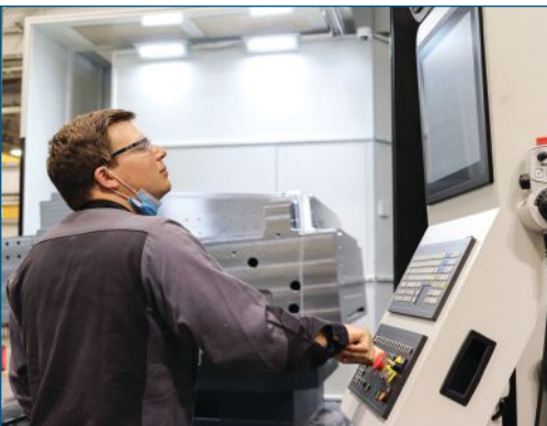
Paragon ordered two CHETO IXN 3000 7-axis milling machines with gundrill ATCs, each equipped to make up to 3-meter/9.8-foot cuts in the X-axis and can hold up to 30-ton workpieces.
