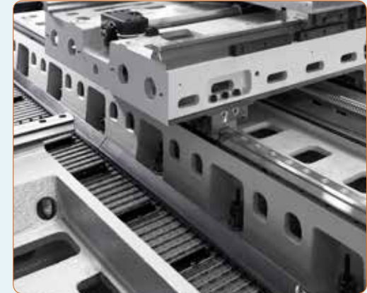
Cast iron structure
