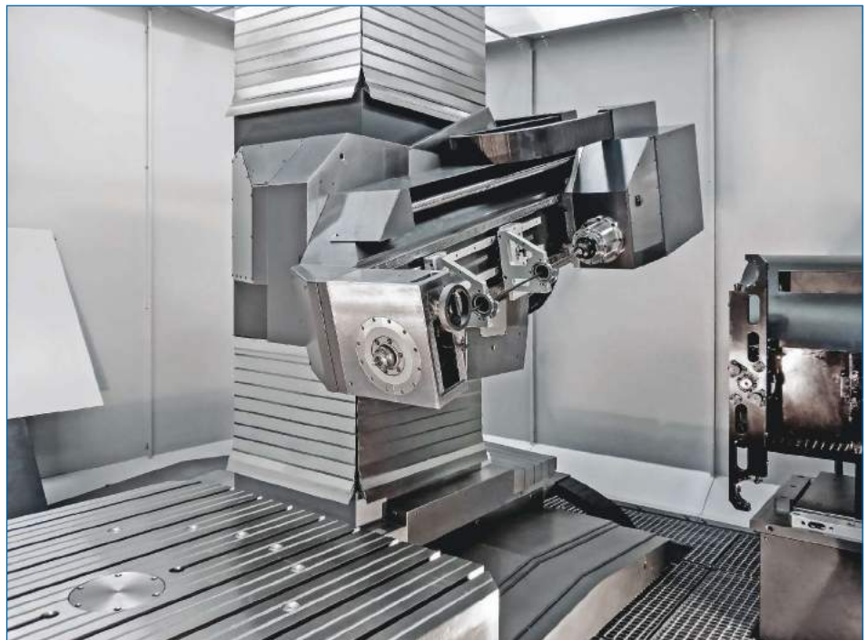
This deep-hole drilling with milling machine from Cheto Corp. S.A. is one of several new, "multi-use" hybrid machining centers, the technologies of which are designed to help moldmakers machine more efficiently and economically.
